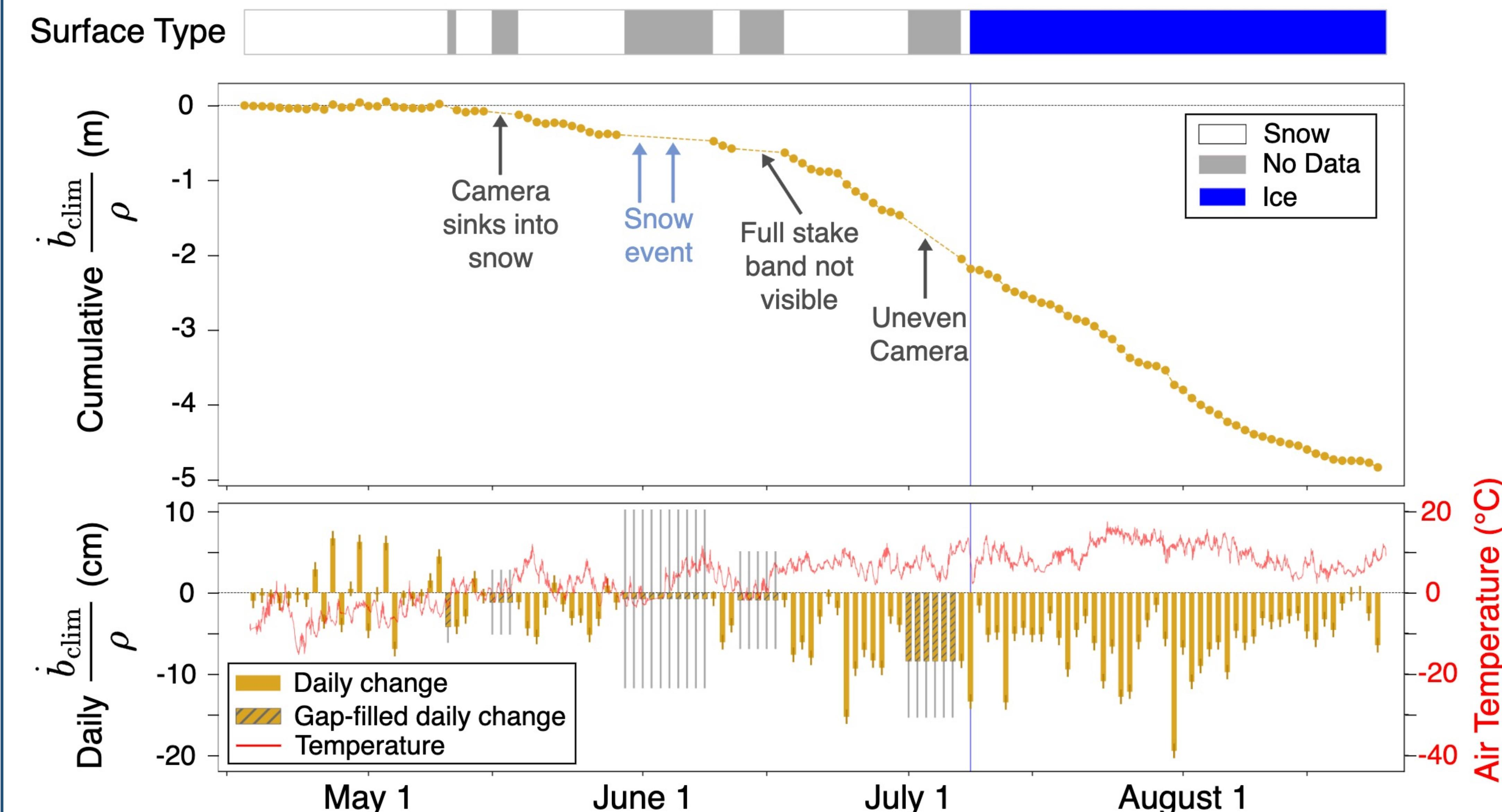
Monitored stake enables continuous mass balance measurements with cm-level accuracy
